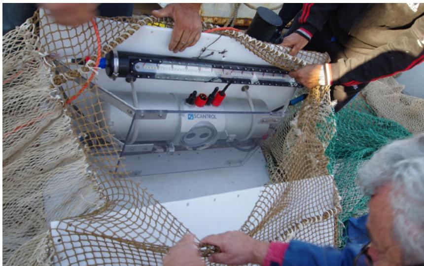
*Figure 5.3.7. Simplified deployment frame used in Greece. The standard Deep Vision camera and lights were mounted inside a frame built on-site using 10 mm thick sheets of high density polyethylene (HDPE).*
