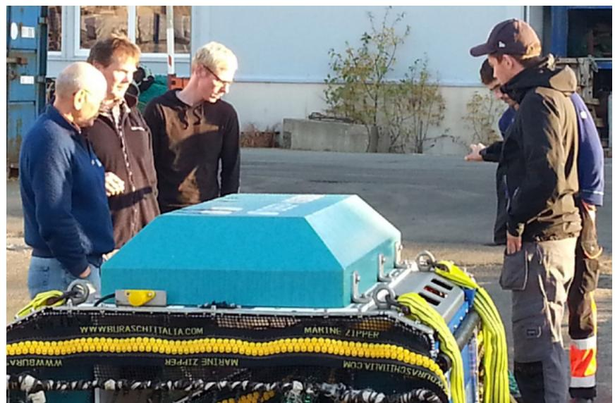
*Figure 5.3.3. Kristoffer Lovall of Scancontrol Deep Vision AS explains the Deep Vision system to the crew of Nergård Havfiske's trawler "Kasfjord" which was docked at the same pier. The yellow SIMRAD transducer used for acoustic transfer is visible in front of the blue floatation block. The yellow zippers were also tested to provide ready access to clean and adjust components inside the frame.*
