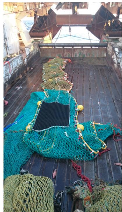
*Figure 5.4.1. The four panel codend with the ExFed system. The picture is taken onboard the trawler "J. Bergvoll".*
