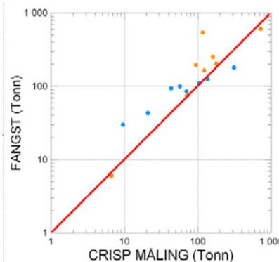
**Figure 5.1.2.** Preliminary summary of verification catches for mackerel and herring schools, using the Simrad SU90 sonar. CRISP Måling (CRISP measurements (tons)), compared with FANGST (CATCH (tons)). The main reason for the more systematic deviation may be incorrect target strength in lateral mode, while larger deviations are either uncertainty (Fig 5.1.3) or error in either catch or measurement.
