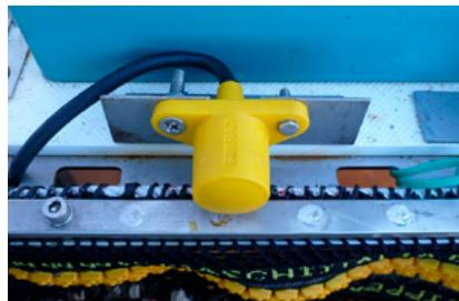
Figure 5.3.5. Simrad transducer mounted to Deep Vision frame for acoustic transfer of system status. Development of the acoustic transfer protocol is being done in cooperation with Kongsberg Simrad.
