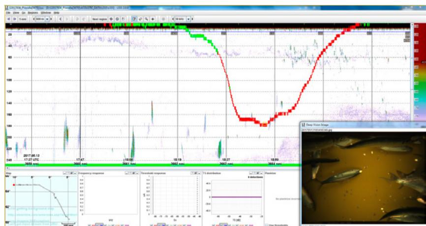
*Figure 5.3.1. Integration of Deep Vision images with LSSS software for analysis of acoustic data. Green and red line traces the trawl's path through the water column (vertical axis = water column depth, horizontal axis = time). The image at lower right is from the position indicated by the small orange box (180 m depth) and provides confirmation that the schools observed are Atlantic herring.*
