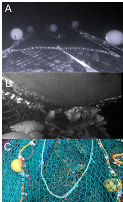
*Figure 5.4.2. A: Underwater photo of the ExFed system, showing the rubber mat. B: Underwater film from the inside of the ExFed system: The smooth inner-lining of the rubber mat can be seen. C: The rear part of the ExFed opening was cut round in a "U" shape.*
