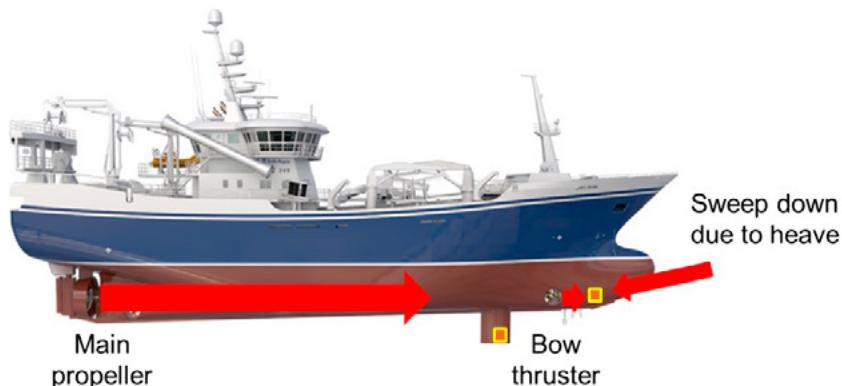
*Figure 5.2.1. Illustration showing the location of the SN90 transducer in the standard position between the bow and the bow thruster, and the new location in the starboard face of the scientific keel. The sources of air bubbles affecting the performance of the hull mounted transducer are indicated by the red arrows.*
