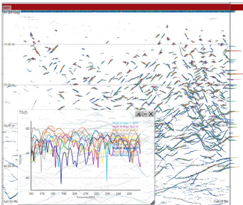
Figure 5.1.7. Example of observations of herring using the probe and WBAT system lowered into a herring layer in Kvænangen in 2017. Note the spectrum of individual targets.
