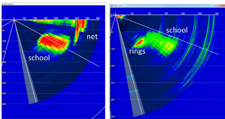
*Figure 5.2.2. Vertical beams of the SN90 sonar during purse seine deployment (left panel) and during pursing (right panel). In the left panel the school can be observed and the net sinking at ca. 300 m range. In the right panel the school can be identified together with the rings from the bottom line, as they approach to the vessel during pursing.*
