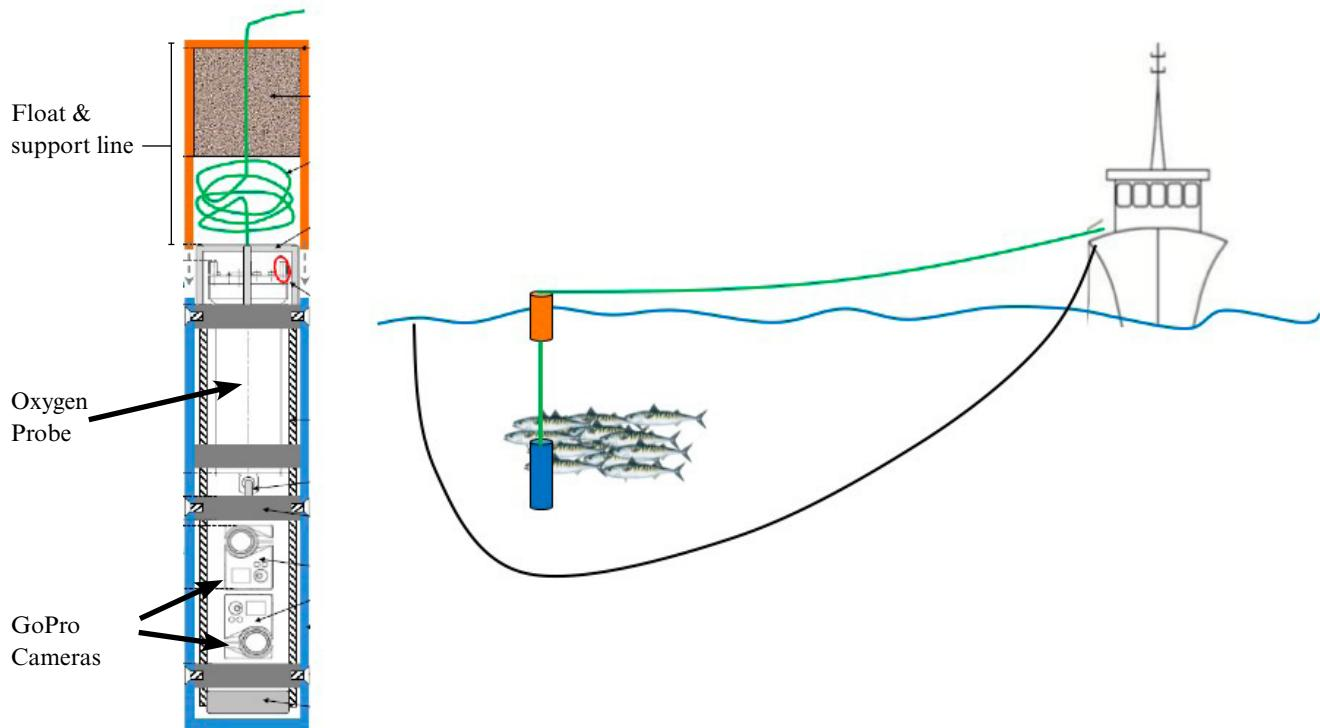
Figure 5.2.4. The catch monitoring probe deployed into a purse seine catch.
