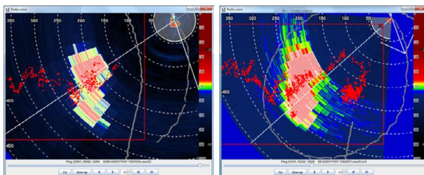
**Figure 5.1.4.** Herring school measured before catch, overserved with the omni sonar SU90 (left panel) and with the in-seine sonar SN90 (right panel). The figures show one simultaneous ping for both sonars. Note the higher number of beams and the higher resolution along each beam in the SN90 sonar.
