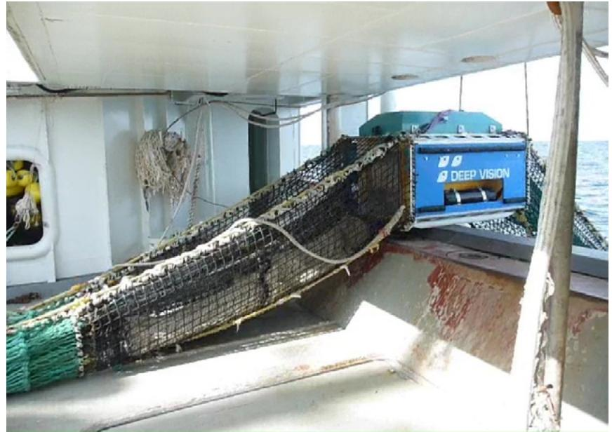
*Figure 5.3.2. Deep Vision system being set out from the commercial trawler / purse seiner MS "Vendla" between Norway and Iceland. The system was successfully deployed on 20 trawl hauls, a total of more than 48 hours of active trawling and image collection.*
