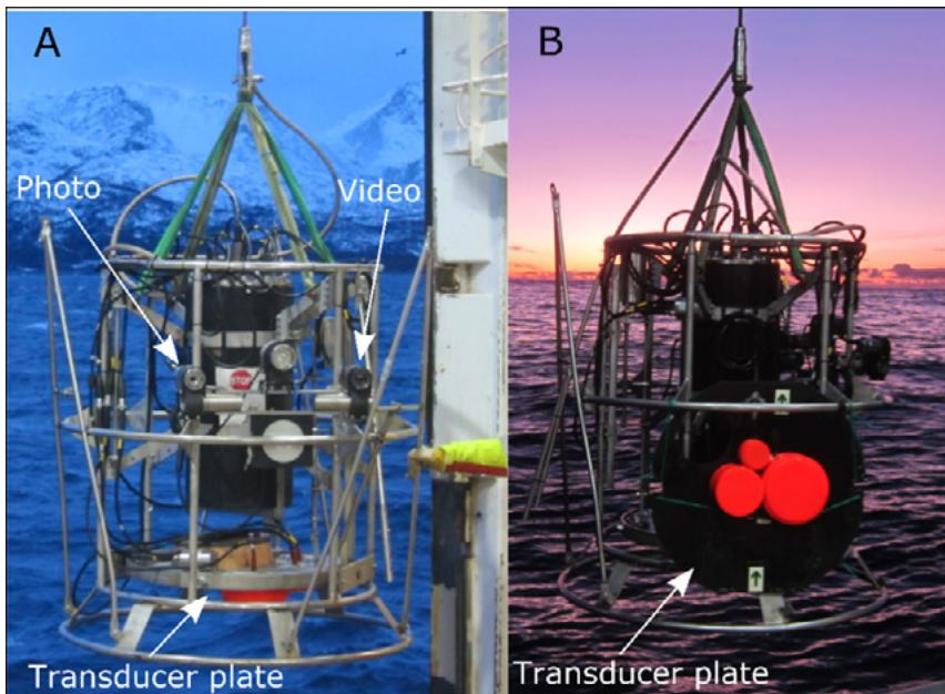
Figure 5.1.6. The TS-probe with transducers mounted for dorsal TS measurements (A) and for lateral aspect TS measurements.
