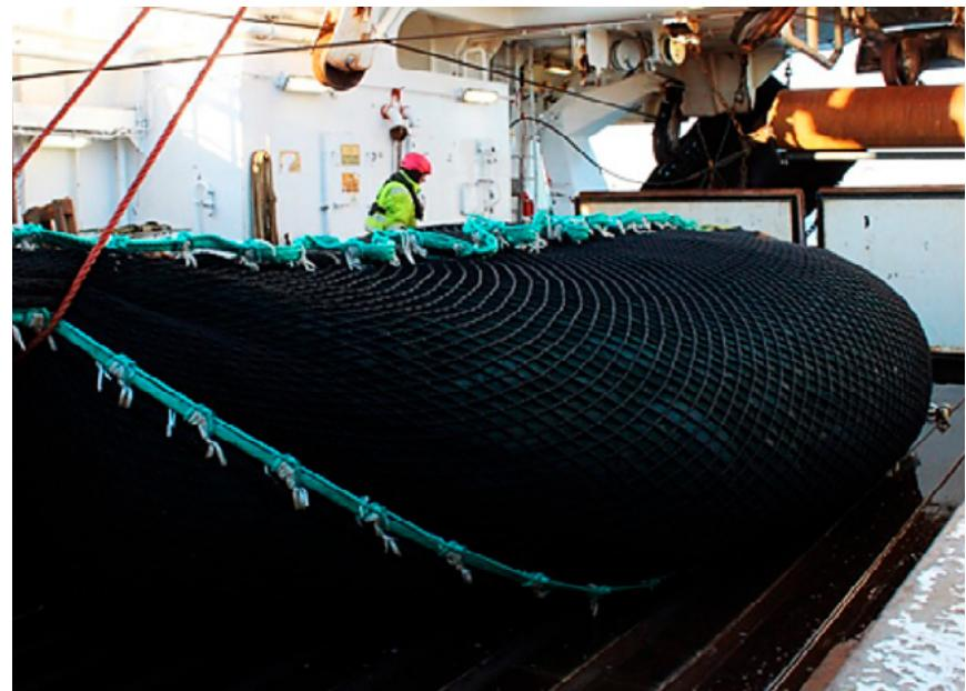
Figure 5.5.6. Testing a new 4-panels codend segment, which is designed in order to improve catch quality. Egersund Group AS, in cooperation with the Institute of Marine Research have designed and built the new codend. The codend segment entrance is closed during towing, not allowing fish to enter, until it reached a predefined depth during haul-back (Photo: Nofima AS).
