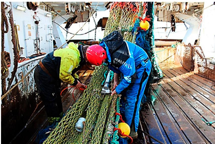
Figure 5.5.8. A hydrostatic codend releaser (FossTech AS) is mounted on top of the commercial trawl codend and releases the fish back into the new codend segment at a given depth (Photo: Nofima AS).
