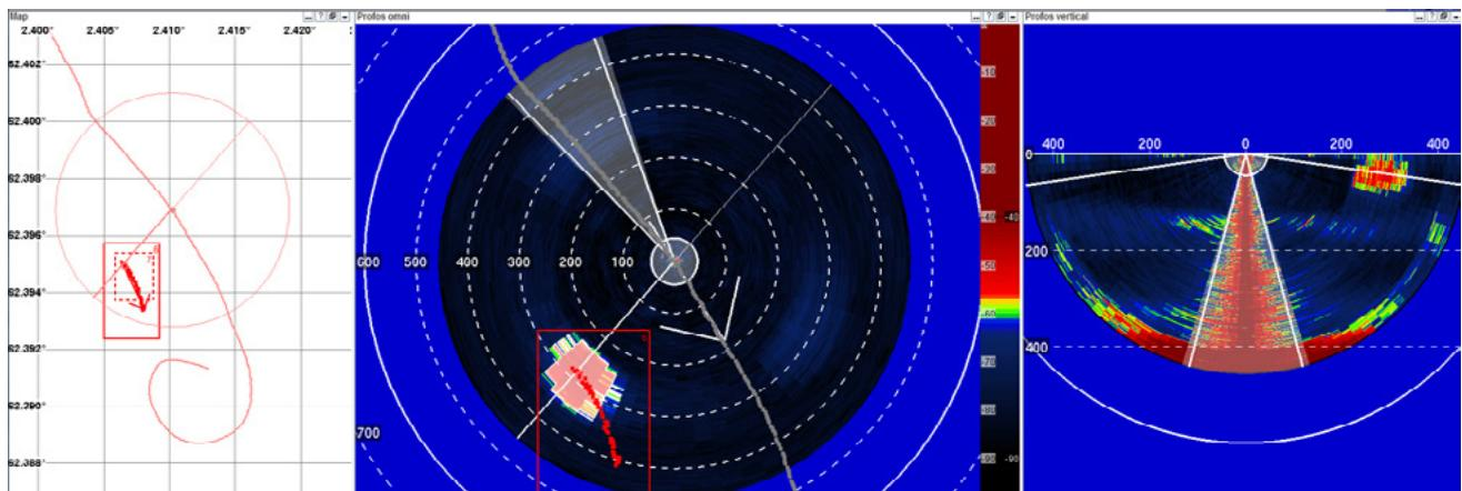
Figure 5.1.1. Detailed skipper inspection of school before catch using the omni sonar SU90. The direction and swimming speed of the school is plotted in the map together with the vessel track (left panel); the horizontal (middle panel) and vertical beams (right panel) are manually adjusted to ensonify the centre of the school for later biomass estimation.
