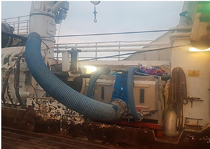
Figure 5.5.4. The new live storage tank installed at the trawl deck onboard FV "J. Bergvoll", Nergård Hayfiske AS (Photo: Nofima AS).
