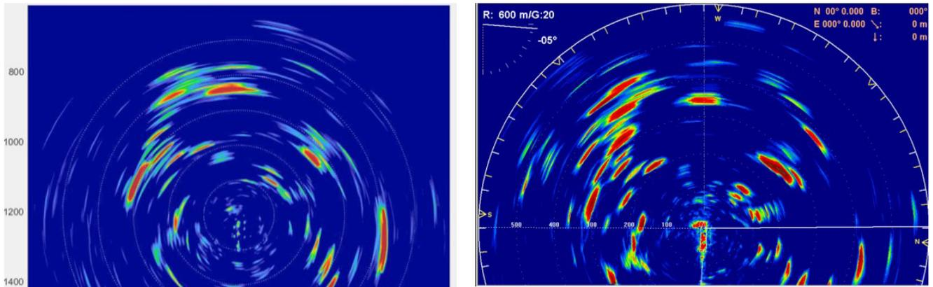
Figure 5.2.2. Display of sonar raw data processed with new developed algorithms (left panel) and screen dump from the sonar display from Simrad SU90 for the same second (right panel).
