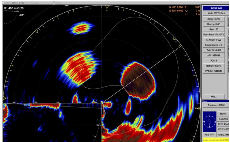
Figure 5.1.1. Dense capelin school where acoustic extinction occur, but not clearly shown in the sonar display. The catch was three times as large as first estimated.
