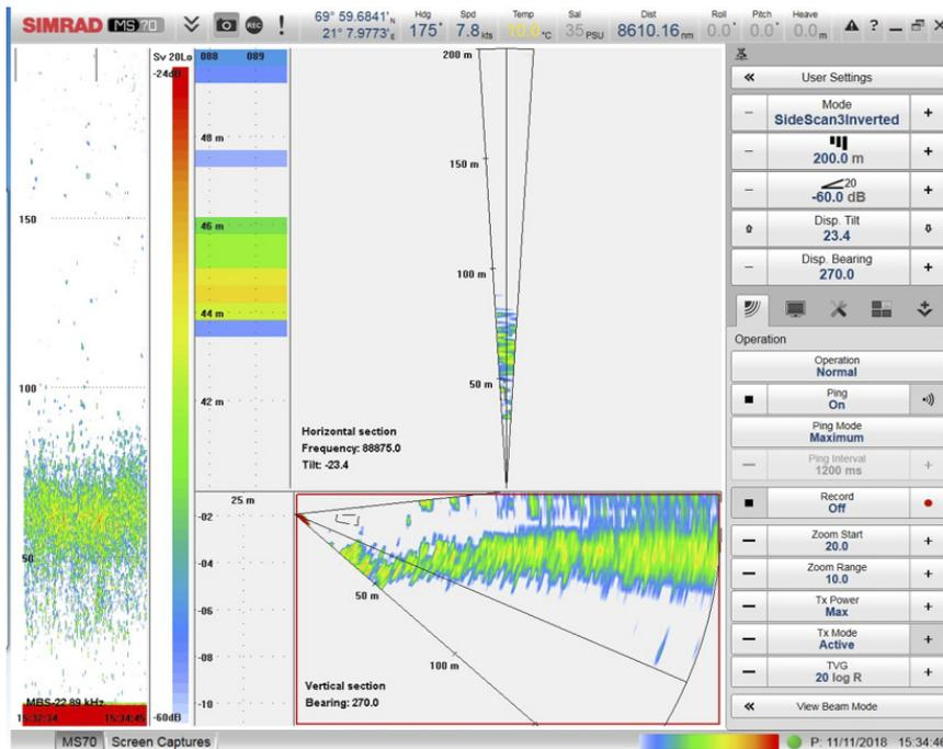
Figure 5.1.3. Measuring herring close to the sea surface with the MS70 sonar.
