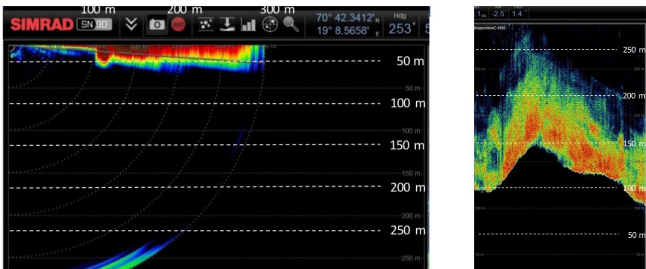
Figure 5.2.1. Vertical section of a capelin school using SN90 sonar with the closer edge of the school at 100 m at a depth of 20 m (left panel). An inspection beam oriented perpendicular to the school, show the decrease (from red to light green colour) in the acoustic backscattering from the closer part of the school at about 100 m towards the distant border about 170 m from the vessel. The range indicates, horizontal distance from the vessel (right panel).
