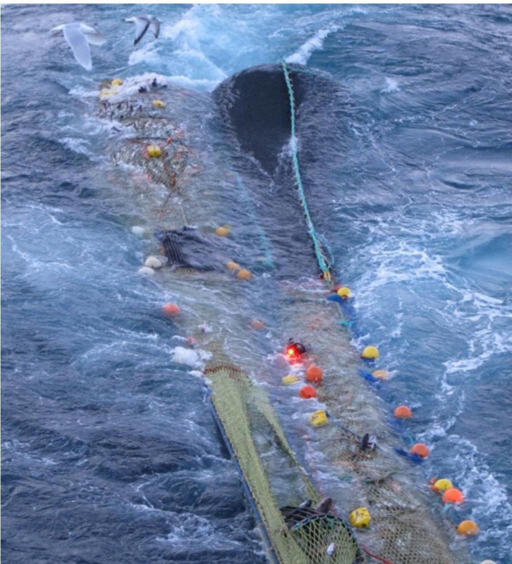
cause a “bucket effect” due to the small mesh size in the improving codend segment, which would cause the fish to stop in the codend with the large mesh size and shrunk lastridges. After a while the fish would fall back into the second codend segment ensuring improved catch quality. The experiments are currently conducted, and the data has not yet been analyzed.
