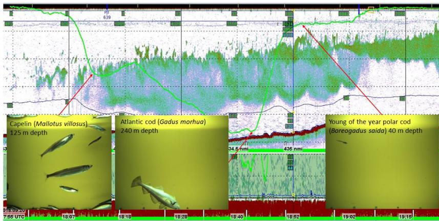
Figure 5.3.7. Composite image showing Deep Vision data (fish images) integrated with acoustic data in LSSS (Large Scale Survey System) software used to analyze acoustic data from the annual Barents Sea ecosystem survey. Deep Vision images confirm that capelin were present in a layer below young-of-the-year polar cod and above adult cod. Image Shale Rosen
