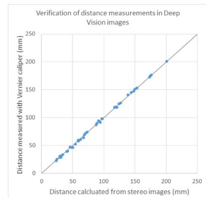
Figure 5.3.4. Distances measured from Deep Vision images ( $x$ -axis) match well with physical measurements made using Vernier caliper. Grey line is expected 1:1 relationship. Fifty-one percent of values were accurate within 1 mm, maximum error was an underestimate by 4.5 mm over a 50 mm interval.
