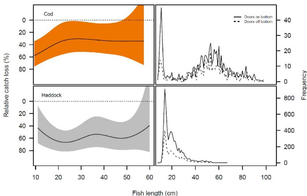
Figure 5.4.1. Left panel: Modelled relative catch loss by fish length for cod (upper) and haddock (lower) when fishing with semi-pelagic rigging as compared to bottom rigging. Right panel: Length frequency distribution for the pooled catch in the eight valid haul pairs.
